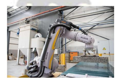
The receiving suction cup, also of particular design, consists of a rectangular plate, capable of supporting horizontal loads up to 360 kg (HEAD INCLUDED)
