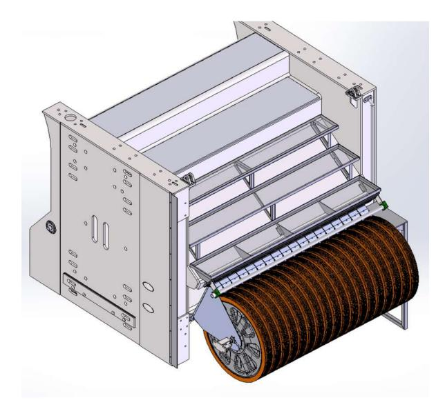
Fig.3 – Detail set of removable free pulleys with pivoting extraction system
