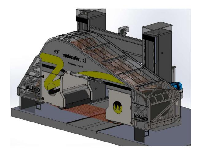
Fig. 5 - Detail of the main frame, housing and protections.
