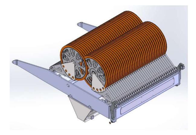
Fig.4 – Detail of the tension pulley assembly, on articulated arms with independent tension cylinders
