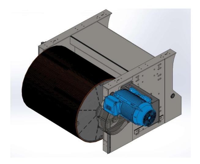
Fig. 2 - Detail of the drum unit, supports and engine transmission.
