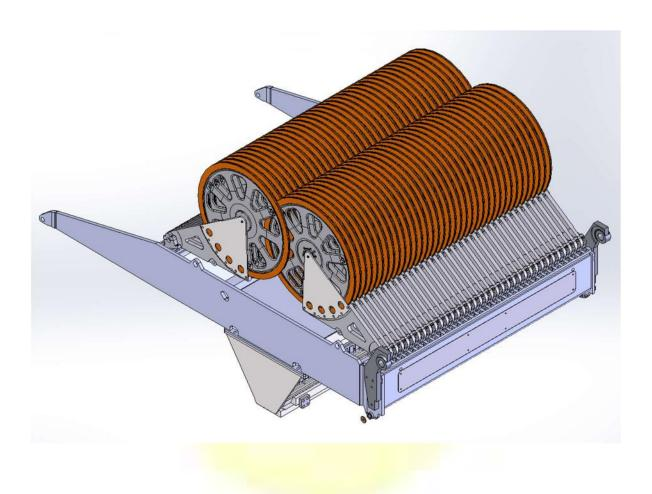
Fig.4 – Detail of the tension pulley assembly, on articulated arms with independent tension cylinders
