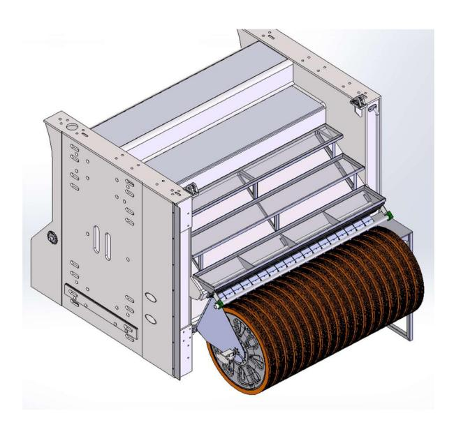
Fig.3 - Detail set of removable free pulleys with pivoting extraction system
