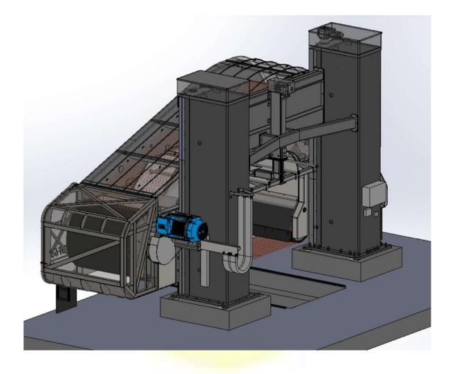
Fig. 6 - Detail of the main frame, columns and crossbar.
