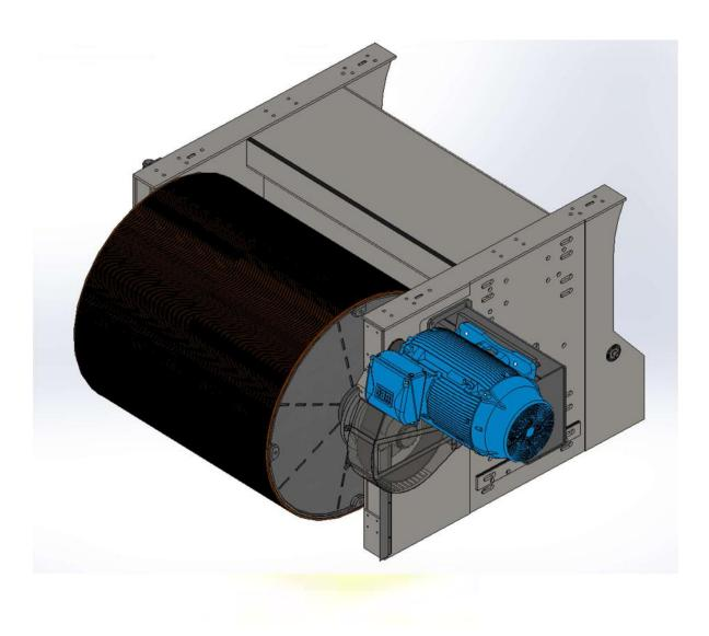
Fig. 2 - Detail of the drum unit, supports and engine transmission.
