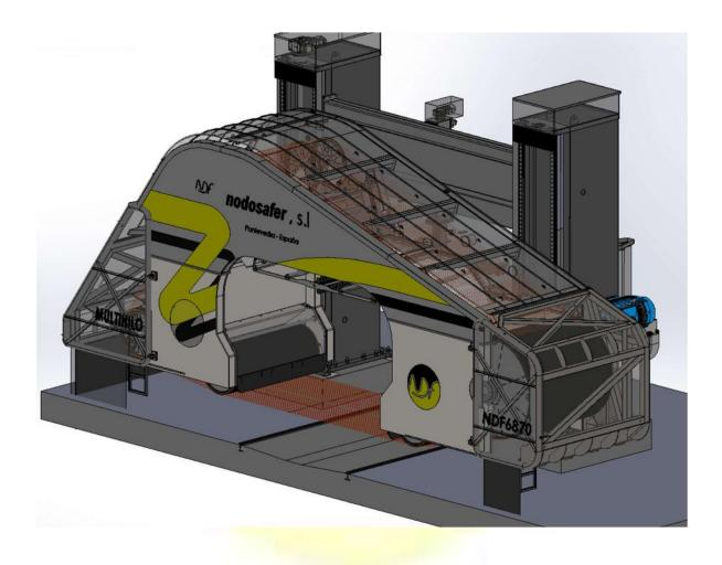
Fig. 5 - Detail of the main frame, housing and protections.
