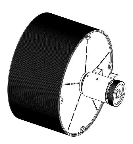
Fig. 4 - Detail of the engine drum unit, support and channels pulley
