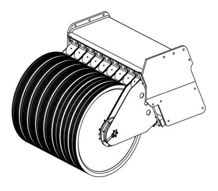
Fig.3 – Detail set of removable free pulleys with pivoting extraction system
