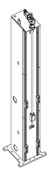
Fig. 1 – Column detail with linear guides, shoes, vertical movement spindles and servomotors
