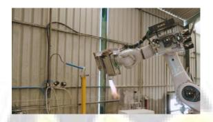
A compact and specially designed head is implemented on the wrist of the Robot, on which the milling motor unit, the torch to perform the buckling, as well as a suction cup for manipulation are based.
